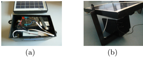
Figure 1: Construction of traffic monitoring unit. Figure 1(a) shows a battery, charging regulator and cameraphone in a steel box while Figure 1(b) shows The box locked and mounted underneath the solar panel
